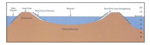
Project islands are below mean sea level because of past subsidence. Reservoir islands would be formed by strengthening island levees, armoring their interior, and constructing intake/outlet pumping facilities.
